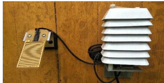
Figure 3. Micro Stations placed on the internal wall of the CLT structure
