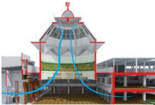
Figure 40: Stack Effect at the Mosque dome
