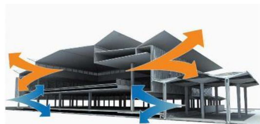
Figure 10: Cross Ventilation design of the Mosque
