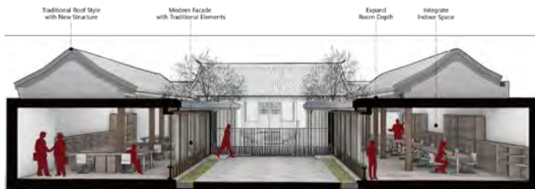
Fig. 27. Adjust the depth of the wing rooms to accommodate commercial functions
