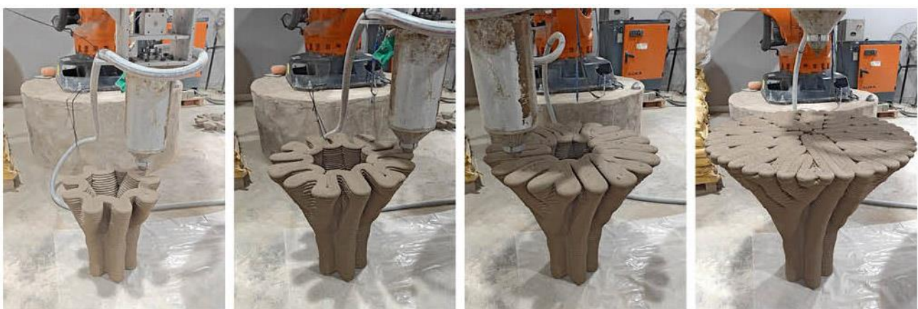
Fig. 9. 3D concrete printing process of the prototype
