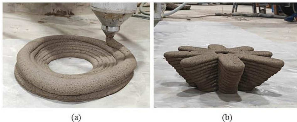
Fig. 4. (a) Initial printing test for shell structure with maximum 50° overhang (b) Initial printing test for rib structure with maximum 50° overhang
