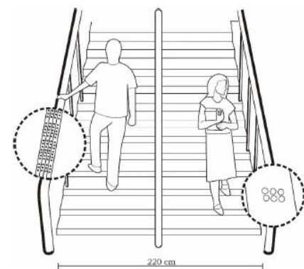
Stairs equipped with braille letters on the top of the handrail at certain intervals indicating the position of the steps (Tactile detail)
