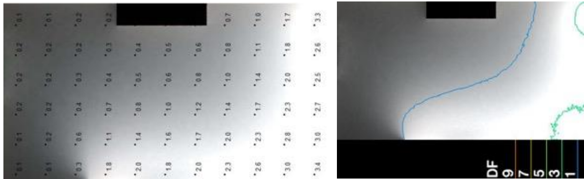
Figure 4: DF results for the main hall area plotted on a 4m x 4m grid & DF contour lines for the main hall area
