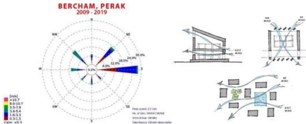
Fig 21. The wind chart of the site with data for the past ten years, and the resulting openings in and within the niche blocks to allow for natural ventilation
