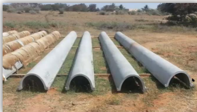
Fig. 10 shows precast Ferrocement Channels placed for curing. Source: Author
