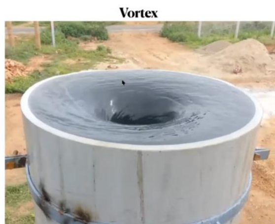
Fig. 20. Vortex for better aeration of the Waste Water. Source: (Gopalan, 2022)
