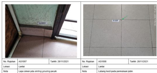
Figure 14 – Defect pictorial evidence of floor defect on ground floor, block A, SMPKVSA.
